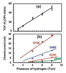
Fig. 6 (a) Turnover frequency for different pressures of  $H_2$  in  $10^5$  Pa of  $O_2$ at 353 K. (b) A plot of the chemicurrent as a function of different H<sub>2</sub> pressures in 10<sup>5</sup> Pa of O<sub>2</sub>. Reprinted with permission from ref. 74. Copyright (2009) American Chemical Society.
