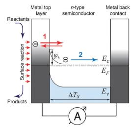
Fig. 7 Temperature gradients and resulting charge carrier transport in a metal-semiconductor nanostructure with  $arphi_{
