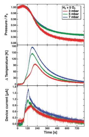
Fig. 8 Pressure, temperature increase and device current observed during the reaction of H2 with O2 in a bulb experiment using a Pt/Si device. The bulb (55l) was filled with  $H_2$  and  $O_2$  in the ratio of 1:5 to total pressures of 3, 5 and 7 mbar. The reaction was initiated at about t = 80 s by irradiating the Pt surface with a light bulb which causes the temperature to rise from room temperature to the ignition temperature.81
