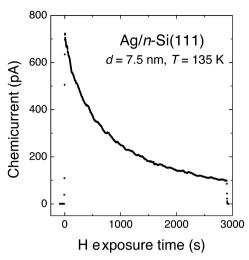
Fig. 4 "Chemicurrent" transient observed by Nienhaus and co-workers when exposing a Ag/n-Si(111) Schottky diode to a flux of H atoms. The device was held at 136 K and the thickness of the Ag layer was 7.5 nm. Adapted from ref. 4 with permission from Elsevier, 2015.
