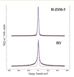
Fig. 1 QENS spectra obtained of methanol loaded in zeolites H-ZSM-5 and HY at Q=0.9 Å at 298 K, (--) represents the resolution data taken at 5 K. The close fit to the resolution function in H-ZSM-5 suggests immobilization, supporting framework methoxylation unlike the significant broadening in HY suggesting intact diffusing methanol.
