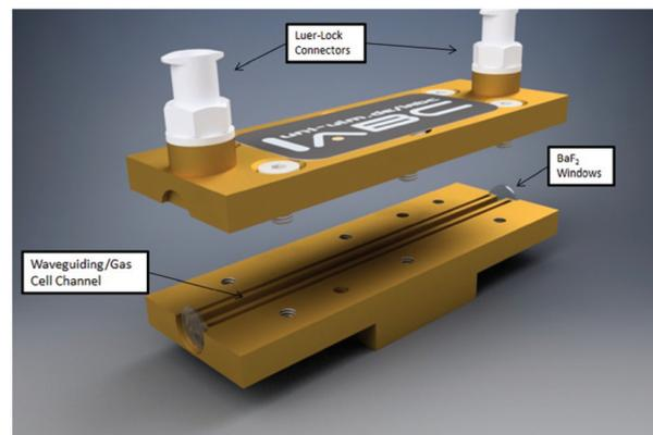
Fig. 2 CAD models of a custom 75 mm long straight-channel iHWG (channel cross-section: 4 mm<sup>2</sup>) equipped with Luer-Lock connectors for gas in/out, and IR-transparent BaF<sub>2</sub> windows sealing the hollow channel for efficient IR radiation in/out coupling.
