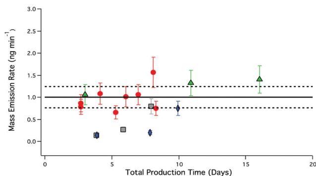
**Fig. 7** PFBA mass emission rate under different RH as a function of total PFBA production time. Red circles, 0% RH; grey squares, 25% RH; blue diamonds, 50% RH; green triangles, 75% RH. Error bars represent the analytical accuracy of the LC-ESI-ToF for each measurement. The solid black line represents the average mass emission rate of PFBA under dry conditions; dashed black lines correspond to the total uncertainty as described in Fig. 5.
