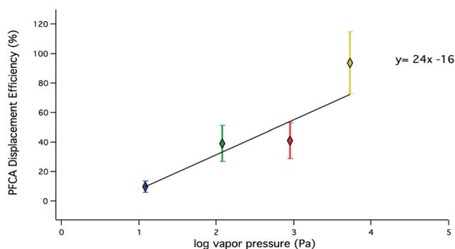
**Fig. 4** PFCA displacement efficiencies under dry conditions as a function of vapour pressure. PFPrA (yellow;  $n = 5$ ), PFBA (red;  $n = 8$ ), PFHxA (green;  $n = 8$ ), PFOA (blue;  $n = 3$ ). Predicted vapour pressures ( $C_4$ – $C_8$ ) are from Bhatarai *et al.*<sup>37</sup> and PFPrA from Sigma Aldrich.<sup>38</sup>
