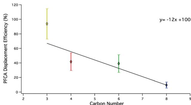
**Fig. 3** Mean displacement efficiencies of PFCA congeners under dry conditions. Error bars represent one standard deviation of congener measurements from each experiment. PFPrA (yellow;  $n = 5$ ), PFBA (red;  $n = 8$ ), PFHxA (green;  $n = 8$ ), PFOA (blue;  $n = 3$ ). The solid black line corresponds to a standard deviation error-weighted linear regression.
