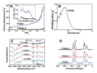
Fig. 2 (A)  $N_2$  sorption isotherm and pore size distribution curve (inset); (B) macropore size distribution, detected using mercury inclusion porosimetry; (C) FT-IR and (D)  $^{13}$ C MAS NMR spectra of the different samples.
