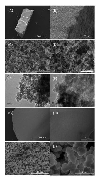
Fig. 1 (A-D) SEM and (E and F) TEM images of PDMBr. SEM images of (G and H) PDMBr-H and (I and J) PDMBr-E.
