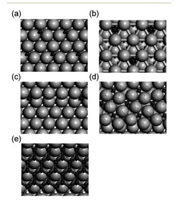
Fig. 20 Different types of adsorbed C atoms on Co surfaces: (a) onsurface; (b) sub-surface; (c) step; (d) P4g clock; (e) graphene. Adapted with permission from ref. 140. Copyright 2010 American Chemical Society.
