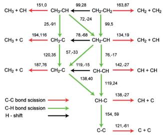
Fig. 6 Reaction barriers and reaction energies (black, first and second values, respectively; in kJ mol<sup>-1</sup>) for various C-H and C-C bondbreaking reactions of ethylene and related species  $C_2H_x$  (x=0-4) over a Pd(111) surface. Reprinted with permission from ref. 88. Copyright 2010 American Chemical Society.
