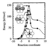
Fig. 10 The calculated energy along the reaction path for  $CH_4$  dissociating over a Ni atom in the Au/Ni(111) surface. The rightmost data points (dashed curves) refer to infinite separation of the dissociated H and  $CH_3$  group on the surface. The dissociation geometry for the three chemical compositions is indicated by the insets, with gold atoms gray-shaded. Reprinted with permission from ref. 37. Copyright 1996 American Institute of Physics Publishing LLC.
