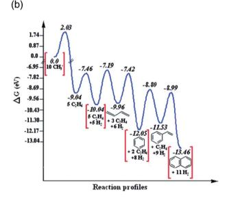
Fig. 18 (a) DFT calculations on catalytic generation of methyl radicals at 1223 K. (b) DFT simulated reaction profile of methyl radicals in the gas phase at 1225 K;  $\Delta G$ , Gibbs free energy. Reprinted with permission from ref. 126. Copyright 2014 American Association for the Advancement of Science.
