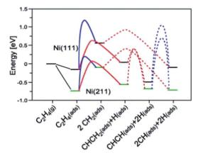
Fig. 7 Potential energy diagram for C-C bond breaking (blue line) and C-H bond breaking (red line) on Ni(111) and Ni(211). The transition state energy for C-H bond breaking of CH<sub>2</sub> is for one CH<sub>2</sub>. Reprinted with permission from ref. 90. Copyright 2006 Elsevier.
