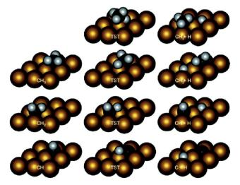
Fig. 2 Intermediate and transition state structures of CH<sub>4</sub> dehydrogenation on Rh(111). Adapted with permission from ref. 52. Copyright 2011 American Chemical Society.
