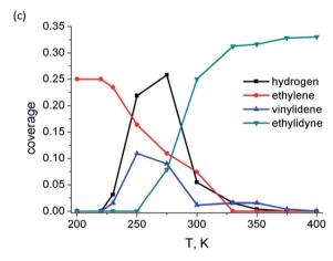
Fig. 5 (a) Reaction network of ethylene transformation over Pt(111); (b) reaction energy profiles (kJ mol<sup>-1</sup>) of vinyl conversion to ethylidyne over Pt(111) at 1/3 coverage (black) and 1/9 coverage (red). Reprinted with permission from ref. 74. Copyright 2010 American Chemical Society; (c) kMC simulated surface coverage after 1 s reaction over Pt(111). Reprinted with permission from ref. 79. Copyright 2012 Elsevier.
