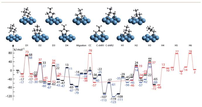
Fig. 9 Structures and energy profiles of the MCP ring-opening reactions over Pt(111): reaction path to 2-methylpentane (2-MP) (black), 3-methylpentane (3-MP) (blue) and nHx (red). Adapted with permission from ref. 95. Copyright 2012 Elsevier.
