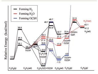
Fig. 15 Lowest-energy pathways of propane ODH process on β-Ga<sub>2</sub>O<sub>3</sub>(100). Reprinted with permission from ref. 116. Copyright 2008 American Chemical Society.
