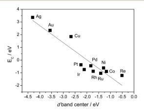
Fig. 3 Relationship between C binding energy and metal d-band center. C binding energies are calculated with  $3 \times 3$  unit cell, BEEF functional. Values of d-band center energies are adapted from ref. 63.
