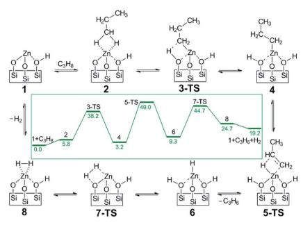
Fig. 19 DFT calculated proposed catalytic reaction pathway for olefin hydrogenation and alkane dehydrogenation on single-site, Zn Lewis acid catalyst. The reaction free energies (kcal mol<sup>-1</sup>) are shown in the inset. Reprinted with permission from ref. 127. Copyright 2014 American Chemical Society.
