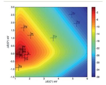
Fig. 4 Two-dimensional volcano-curve of the turnover frequency (log<sub>10</sub>, at 773 K, 1 bar) as a function of C and O binding energy. Reprinted with permission from ref. 7. Copyright 2008 Elsevier.
