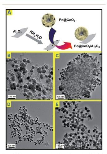
Fig. 4 (A) Schematic representation of the self-assembly of Pd@CeO $_2$  and commercial  $\gamma$ -Al $_2O_3$ ; (B) TEM images of 11 nm-Pd@CeO $_2$ /Al $_2O_3$ ; (C) 13 nm-Pd@CeO $_2$ /Al $_2O_3$ ; (D) 17 nm-Pd@CeO $_2$ /Al $_2O_3$ ; (E) 8 nm-Pd@CeO $_2$ /Al $_2O_3$ .
