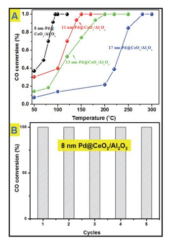
Fig. 6 (A) catalytic CO conversion of  $Pd@CeO_2/Al_2O_3$  with different Pd core sizes; (B) cycling test of 8 nm- $Pd@CeO_2/Al_2O_3$ .
