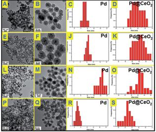
Fig. 2 TEM images and particle size distributions of Pd@CeO $_2$  core@shell nanospheres obtained by addition of different amounts of KBr in the reaction solution: (A), (B), (C) and (D) 150 mg KBr, 50  $\mu$ L NH $_3$ ·H $_2$ O; (E), (F), (J) and (K) 300 mg KBr, 50  $\mu$ L NH $_3$ ·H $_2$ O; (L), (M), (N) and (O) 500 mg KBr, 50  $\mu$ L NH $_3$ ·H $_2$ O; (P), (Q), (R) and (S) 300 mg KBr, 200  $\mu$ L NH $_3$ ·H $_2$ O.
