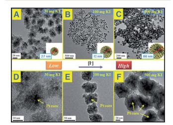
Fig. 3 TEM images of Pt@CeO<sub>2</sub> multi-core@shell nanospheres prepared by KI assistance; (A) and (D): 30 mg; (B) and (E): 100 mg; (C) and (F): 500 mg.
