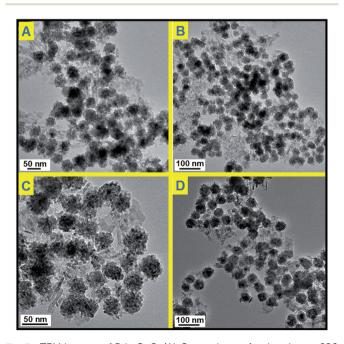
Fig. 5 TEM images of Pd@CeO $_2$ /Al $_2$ O $_3$  products after heating at 600  $^{\circ}$ C for 3 hours; (A) 11 nm; (B) 13 nm; (C) 17 nm; (D) 8 nm.
