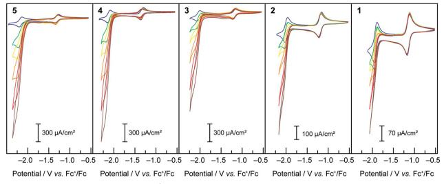
Fig. 2 Cyclic voltammograms under Ar at 50 mV s<sup>-1</sup> of 1 mM solutions of compounds 1–5 in DMF, TBAPF6 0.1 M, on a glassy carbon electrode with 0 (— blue), 5 (— green), 10 (— yellow), 20 (— orange), 40 (— red) and 60 (— brown) mM of acetic acid.
