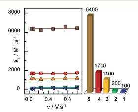
Fig. 4 Left:  $k_1$  values obtained through the *FOWA* of compounds 1 ( blue), 2 (— green), 3 (— orange), 4 (— red) and 5 (— brown) at different scan rates. Right: corresponding  $TOF_{max}$  (in  $s^{-1}$ ) for an acid concentration of 1 M.
