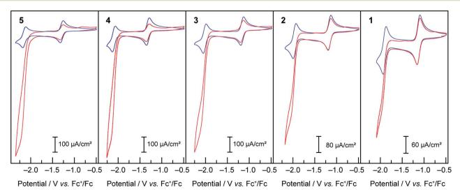
Fig. 6 Cyclic voltammograms under Ar (— blue) and  $CO_2$  (— red) at 50 mV s<sup>-1</sup> of 1 mM solutions of compounds 1–5 in DMF/H<sub>2</sub>O (95 : 5), TBAPF<sub>6</sub> 0.1 M.
