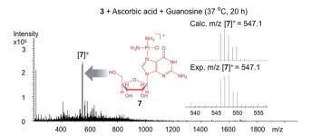
Fig. 3 ESI-MS of the reaction mixture of 3 (0.16 mM), ascorbic acid (17 mM), and guanosine (0.62 mM). The cationic adduct 7 forms from the reaction of the released cisplatin and guanosine.
