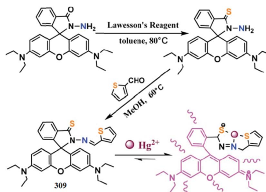
Fig. 271 Synthetic route, molecular structure and \text{Hg}^{2+} binding mode of ligand 309 .
