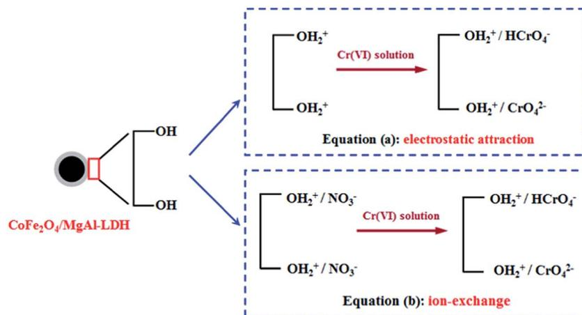
Fig. 8 Schematic illustration of the adsorption mechanism of Cr(vi) on CoFe<sub>2</sub>O<sub>4</sub>/MgAl-LDH.
