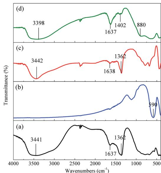
Fig. 6 FTIR spectra of (a) MgAl-LDH, (b) CoFe<sub>2</sub>O<sub>4</sub>, (c) CoFe<sub>2</sub>O<sub>4</sub>/MgAl-LDH, (d) CoFe<sub>2</sub>O<sub>4</sub>/MgAl-LDH after Cr(vi) adsorption.
