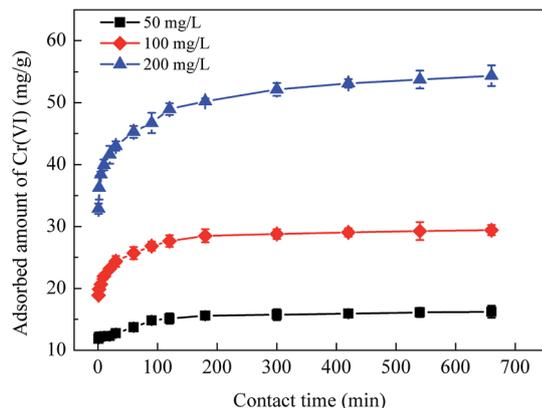
Fig. 3 Effect of contact time on Cr(vi) adsorption using CoFe<sub>2</sub>O<sub>4</sub>/MgAl-LDH for initial Cr(vi) concentrations of 50, 100 and 200 mg L<sup>-1</sup>.
