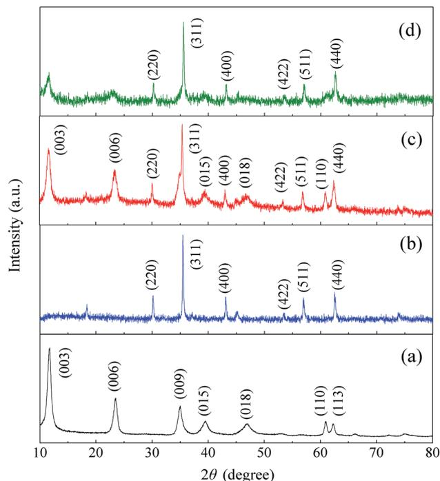
**Fig. 1** XRD patterns of (a) MgAl-LDH, (b) CoFe<sub>2</sub>O<sub>4</sub>, (c) CoFe<sub>2</sub>O<sub>4</sub>/MgAl-LDH, and (d) CoFe<sub>2</sub>O<sub>4</sub>/MgAl-LDH after Cr(vi) adsorption.
