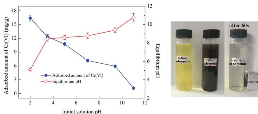
**Fig. 2** Effect of initial solution pH on Cr(vi) adsorption and equilibrium pH using CoFe<sub>2</sub>O<sub>4</sub>/MgAl-LDH.
