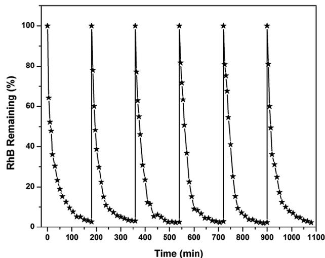
Fig. 7 Reusable nature of magnetite for the electro Fenton oxidation of rhodamine B. Figure taken from ref. 80.
