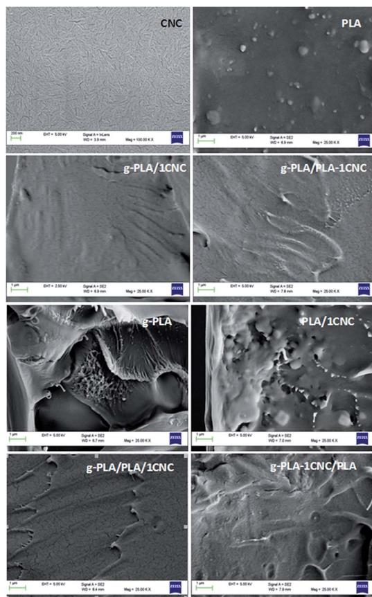
Fig. 5 FESEM images of cellulose nanocrystals (CNC) and fractured samples of neat PLA, g-PLA and PLA nanocomposite systems obtained by different masterbatch procedures.
