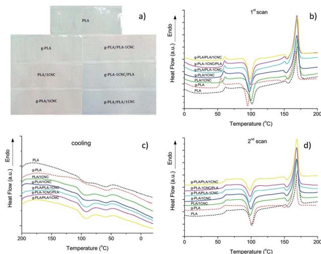
Fig. 2 Visual appearance of films (a), DSC thermograms related to the (b) first heating scan, (c) cooling scan and (d) second heating scan of neat PLA, g-PLA and PLA nanocomposite systems obtained by different masterbatch procedures.
