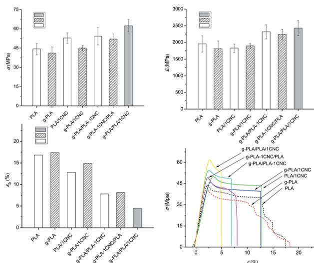
Fig. 4 Values for tensile strength (a), Young's modulus (b), elongation at break (c) and stress-strain curves for neat PLA, g-PLA and PLA nanocomposite systems (d) obtained by different masterbatch procedures.
