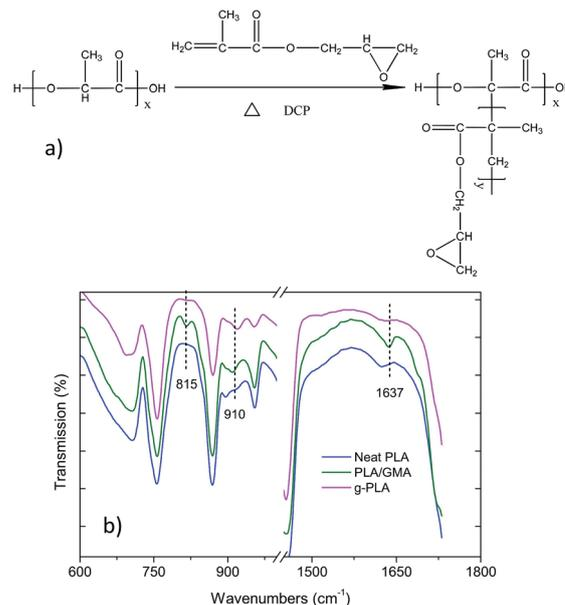
Fig. 1 (a) Mechanism of the grafting of GMA onto the PLA chain and (b) FTIR spectra of neat PLA, PLA/GMA, and g-PLA.
