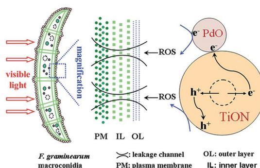
Fig. 7 Photocatalytic disinfection mechanism of  $\text{TiON}/\text{PdO}$  photocatalyst on *Fusarium graminearum* macroconidia under visible light irradiation. Reproduced with permission from ref. 157, copyright (2013) American Chemical Society.
