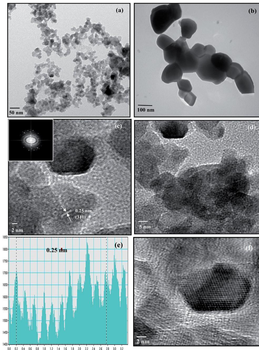
**Fig. 1** TEM images of  $\text{CuFe}_2\text{O}_4$  annealed at (a) 400 °C and (b) 1000 °C, HRTEM images of the  $\text{CuFe}_2\text{O}_4$  nanoparticles at (c) magnification of 2 nm (inset shows the FFT of  $\text{CuFe}_2\text{O}_4$ ) and (d) magnification of 5 nm. (e) Frame profile for the average fringe width. (f) Reconstructed image after filtering the FFT pattern from HRTEM.
