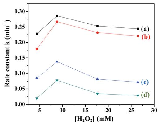
Fig. 9 Variation of rate constants with [H<sub>2</sub>O<sub>2</sub>] in the presence of (a) CuFe<sub>2</sub>O<sub>4</sub>, (b) ZnFe<sub>2</sub>O<sub>4</sub>, (c) NiFe<sub>2</sub>O<sub>4</sub> and (d) CoFe<sub>2</sub>O<sub>4</sub>.
