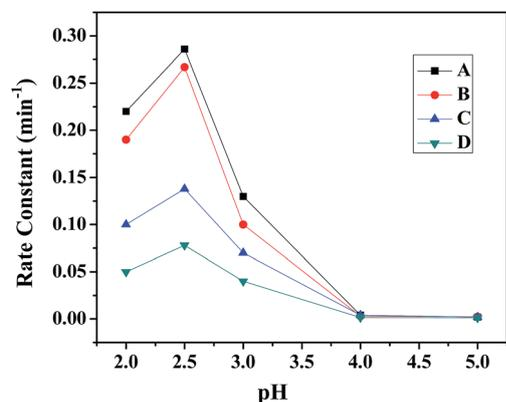
Fig. 10 Effect of pH on the rate constant in the presence of (A) CuFe<sub>2</sub>O<sub>4</sub>, (B) ZnFe<sub>2</sub>O<sub>4</sub>, (C) NiFe<sub>2</sub>O<sub>4</sub> and (D) CoFe<sub>2</sub>O<sub>4</sub>.
