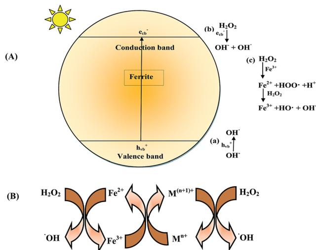
Fig. 12 (A) Mechanism of generation of a hydroxyl radical ( $\text{OH}^\cdot$ ) in the presence of a ferrite/ $\text{H}_2\text{O}_2$ /light system. (B) General mechanism of electron transfer occurring in ferrite.
