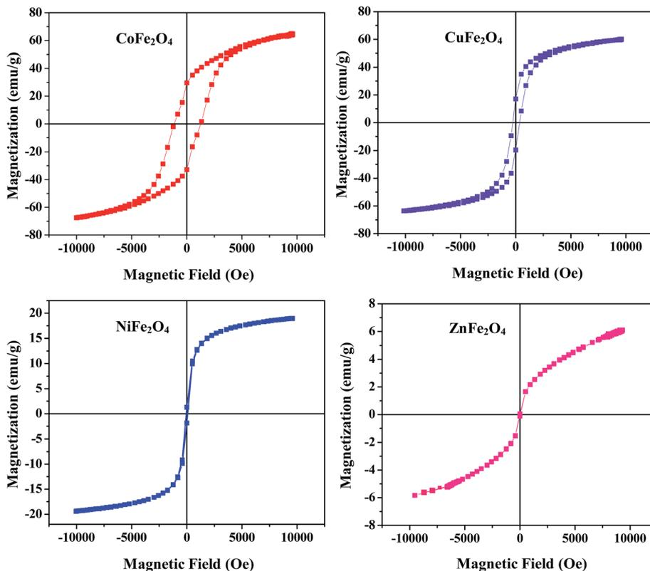
Fig. 4 Magnetic hysteresis loops for the ferrites annealed at 400 °C.
