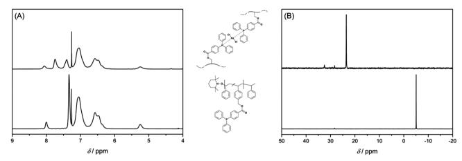
Fig. 1 Intramolecular crosslinking by metal-ligand complexation monitored by <sup>1</sup>H NMR (A) and <sup>31</sup>P{<sup>1</sup>H} NMR spectroscopy (B) in CDCl<sub>3</sub> at 25 °C. The complete shift of the proton and phosphorus resonances indicates quantitative complexation (the crosslinking chemistry presents a schematic view, in which we suggest a *trans*-configuration of the Pd-atoms, see text).
