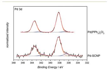
Fig. 5 Pd 3d XPS spectra of Pd-SCNP (bottom) and [Pd(PPh<sub>3</sub>)<sub>2</sub>Cl<sub>2</sub>] (top). The comparison of the prepared SCNPs with the model complex shows that the binding energy of the main Pd species at 338.2 eV in Pd-SCNP is in excellent agreement with the binding energy in [Pd(PPh<sub>3</sub>)<sub>2</sub>Cl<sub>2</sub>].
