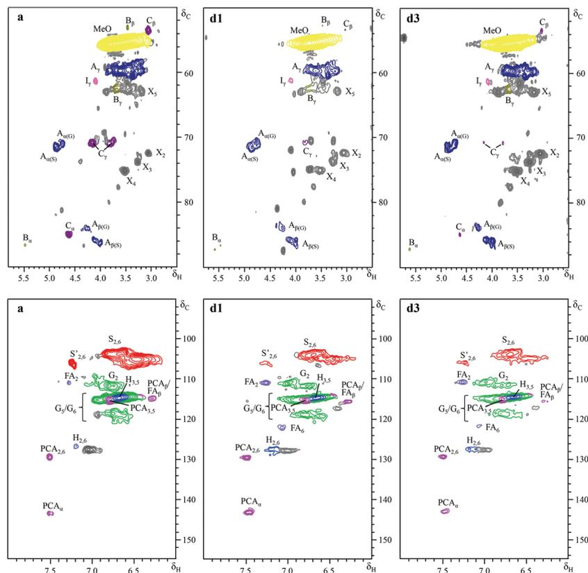
**Fig. 4** Side chain ( $\delta_C/\delta_H$  50–90/2.5–5.8) and aromatic/unsaturated ( $\delta_C/\delta_H$  90–155/5.5–8.0) regions in the 2D HSQC NMR spectra of (a) P1000 soda lignin, (d1) after extraction sequence NH<sub>3</sub>/DCM the NH<sub>3</sub> is at 7 bars autogeneous pressure and at 18 °C, and (d3) after extraction sequence NH<sub>3</sub>/DCM (at 90 bars total pressure of NH<sub>3</sub> and hydrogen and at 85 °C).
