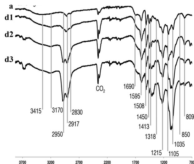
**Fig. 3** FT-IR spectra of (a) soda P1000 lignin, (d1) after extraction sequence NH<sub>3</sub>/DCM (the NH<sub>3</sub> is at 7 bars autogeneous pressure and at 18 °C), (d2) after extraction sequence NH<sub>3</sub>/DCM (at 90 bars total pressure of NH<sub>3</sub> and argon and at 85 °C) and (d3) after extraction sequence NH<sub>3</sub>/DCM (at 90 bars total pressure of NH<sub>3</sub> and hydrogen and at 85 °C).
