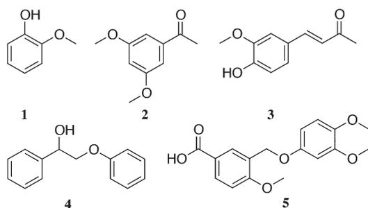
**Fig. 2** Main monomers and dimers extracted after solubilisation in ammonia (a full list is included in the ESI<sup>†</sup>): (1) guaiacol; (2) 2,5-dimethoxyacetophenone; (3) vanillideneacetone; (4) 2-phenoxy-1-phenylethanol and (5) 3-((3,4-dimethoxyphenoxy)methyl)-4-methoxybenzoic acid.
