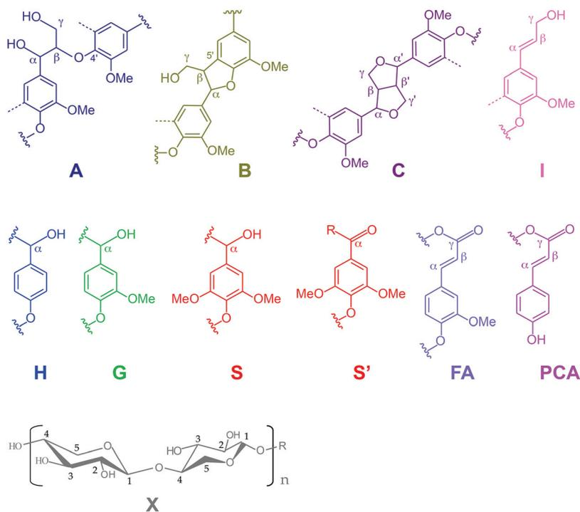
**Fig. 5** Main structures present in the (treated) P1000 soda lignins: (A)  $\beta$ –O-4' alkyl–aryl ethers; (B)  $\beta$ –5' phenylcoumarans; (C)  $\beta$ – $\beta'$  resinols; (I) cinnamyl alcohol end groups; (H) *p*-hydroxyphenyl units; (G) guaiacyl units; (S) syringyl units; (S') syringyl units bearing a carbonyl group in position  $\alpha$ ; (PCA) *p*-coumarates; (FA) ferulates and (X) xylans.
