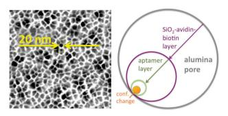
Fig. 3 Left: SEM picture of pore-structure of the AAO-membrane with a nominal pore size of 20 nm in its pristine form; right: schematic on the effect of the gradual membrane surface modifications on the effective pore-size.
