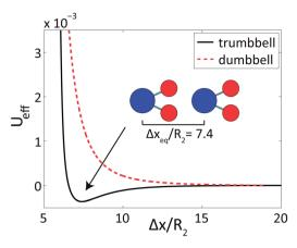
Fig. 6 Effective potentials for two dumbbells (dashed red line) and two trumbbells (solid black line) aligned in the flow direction in unbounded g2D. The quadrupolar contribution to the interaction of two dumbbells is repulsive. For two trumbbells, the quadrupolar component is attractive. Higher order, shorter range multipole components are repulsive, stabilizing the trumbbells against collision. As a result, two trumbbells have an equilibrium separation  $\Delta x_{eq}/R_2 = 7.4$ .
