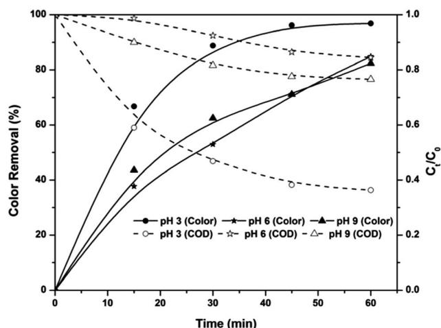
Fig. 3 Effect of solution pH on color and COD removal kinetics of the EF process at an applied voltage of 7 V and ferric ion concentration of 10 mg L<sup>-1</sup>.
