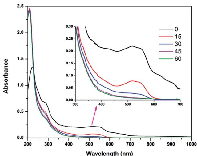
Fig. 6 Changes in UV-visible spectra of textile wastewater at applied voltage of 7 V, pH 3 and ferric ion concentration of 10 mg L<sup>-1</sup>.
