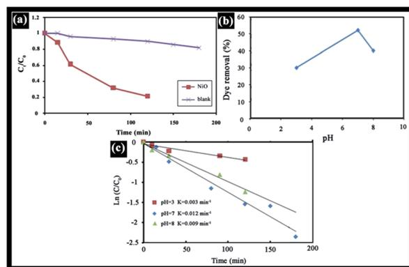
Fig. 8 (a) Variation in RB concentration with time (NiO dose ( $W$ ) =  $1 \text{ g L}^{-1}$ ,  $[\text{RB}] = 10 \text{ mg L}^{-1}$ ,  $\text{pH} = 7$ ), (b) pH effect on the removal of RB dye (NiO dose ( $W$ ) =  $1 \text{ g L}^{-1}$ ,  $[\text{RB}] = 10 \text{ mg L}^{-1}$ ,  $T = 20 \text{ }^\circ\text{C}$ ,  $t = 12 \text{ h}$ ), (c) effect of the initial pH on the photocatalytic degradation of RB dye (NiO dose ( $W$ ) =  $1 \text{ g L}^{-1}$ ,  $[\text{RB}] = 10 \text{ mg L}^{-1}$ ).
