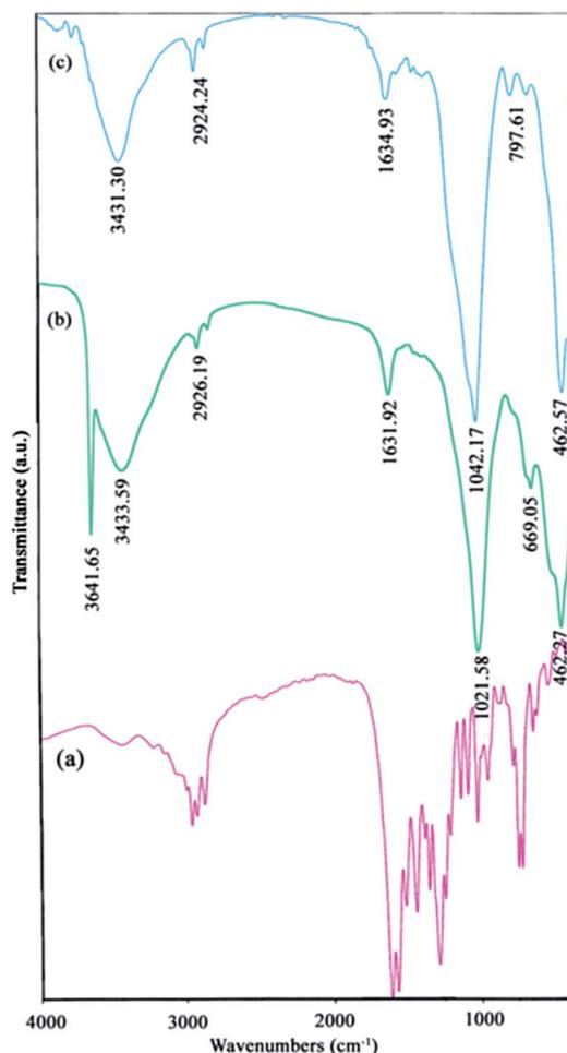
Fig. 1 FT-IR spectra of (a) H<sub>2</sub>(pnAA<sub>2</sub>), (b) β-Ni(OH)<sub>2</sub>, and (c) calcinated NiO at 750 °C.
