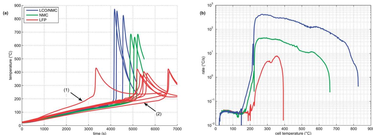
**Fig. 5** (a) Overview of the time–temperature profiles for the cells tested. Data for the whole experiment durations and for the whole experiment sets is shown. For the sake of completeness, one LFP test with a higher (1) and one with a lower (2) heating rate of the heater sleeve are included. (b) Temperature rates from three representative experiments.
