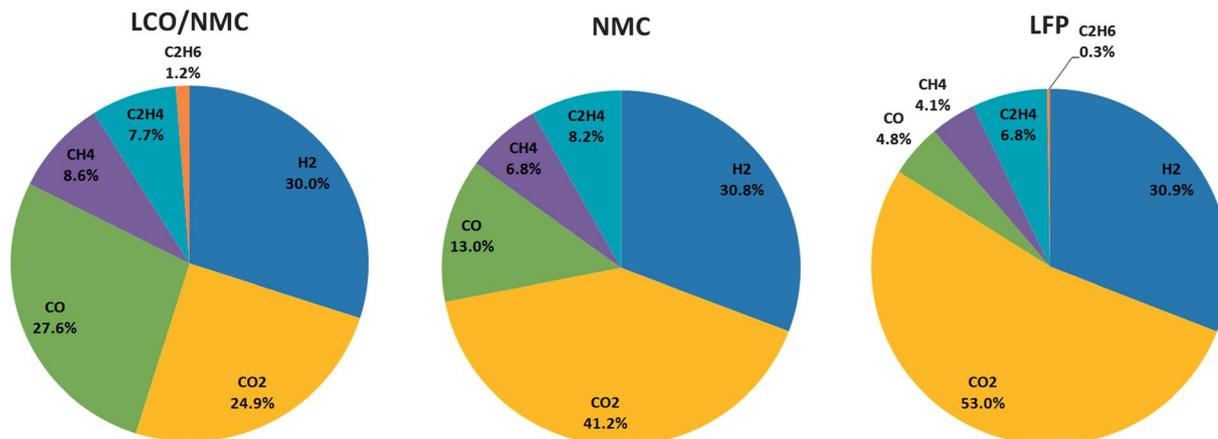
Fig. 6 Detected components of the produced gases (mol%).
