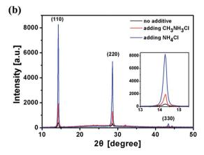
Fig. 2 UV-vis absorption spectra (a) and XRD patterns (b) for  $CH_3NH_3PbI_3$  films fabricated by using different additives.
