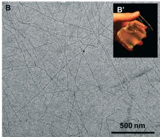
Fig. 1 a) Optical micrograph of TEMPO-oxidized cellulose fiber; b) TEM of the TEMPO-oxidized cellulose fiber. 44 Reprinted with permission from T. Saito, M. Hirota, N. Tamura, S. Kimura, H. Fukuzumi, L. Heux, A. Isogai, Individualization of nano-sized plant cellulose fibrils by direct surface carboxylation using TEMPO catalyst under neutral conditions, Biomacromolecules, 2009, 10(7), 1992-1996. Copyright 2014 American Chemical Society.
