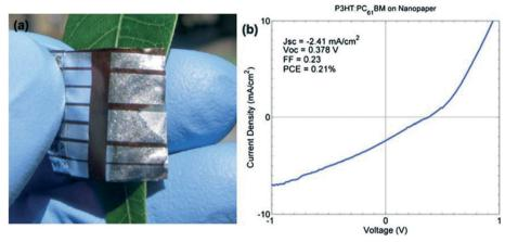
Fig. 5 Printed solar cells on transparent and conductive nanopaper. (a) An organic solar cell on conductive nanopaper. (b) The I-V curve of the organic solar cell shown in (a). 65 Reproduced from L. Hu, G. Zheng, J. Yao, N. Liu, B. Weil, M. Eskilsson, E. Karabulut, Z. Ruan, S. Fan, J. T. Bloking, Transparent and conductive paper from nanocellulose fibers, Energy Environ. Sci., 2013, 6(2), 513-518. With permission from The Royal Society of Chemistry. Copyright 2014 The Royal Society of Chemistry.
