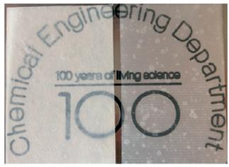
Fig. 2 Comparison of the transparent papers made from BC (left) and MFC (right).<sup>33</sup> Reprinted with permission from K. Y. Lee, T. Tammelin, K. Schulfter, H. Kiiskinen, J. Samela, A. Bismarck, High performance cellulose nanocomposites: comparing the reinforcing ability of bacterial cellulose and nanofibrillated cellulose, ACS Appl. Mater. Interfaces, 2012, 4(8), 4078-4086. Copyright 2014 American Chemical Society.
