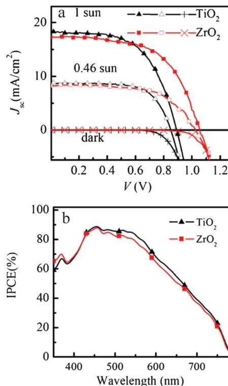
**Fig. 3**  $J$ - $V$  curve in the dark and under AM 1.5G illumination of  $1000 \text{ W m}^{-2}$  and  $460 \text{ W m}^{-2}$  intensity. IPCE spectra of spiro-OMeTAD/ $\text{CH}_3\text{NH}_3\text{PbI}_3/\text{ZrO}_2$  and spiro-OMeTAD/ $\text{CH}_3\text{NH}_3\text{PbI}_3/\text{TiO}_2$  solar cell.
