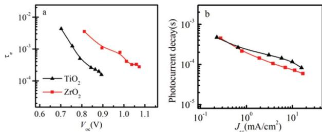
**Fig. 5** (a) Electron lifetime as a function of open circuit voltage in spiro-OMeTAD/CH<sub>3</sub>NH<sub>3</sub>PbI<sub>3</sub>/ZrO<sub>2</sub> (or TiO<sub>2</sub>) solar cells. (b) Photocurrent transient decay as a function of short-circuit current in spiro-OMeTAD/CH<sub>3</sub>NH<sub>3</sub>PbI<sub>3</sub>/ZrO<sub>2</sub> (or TiO<sub>2</sub>) solar cells.
