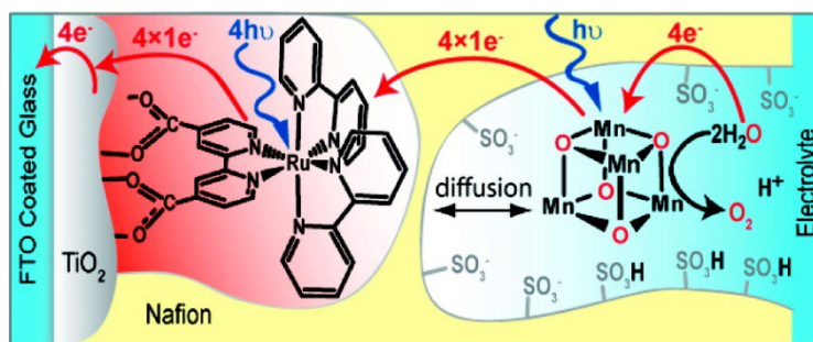
Figure 22. Schematic depiction of the photoelectrochemical cell containing Mn cubane 40 . Reprinted with permission from ref. 160. Copyright 2010 American Chemical Society.
