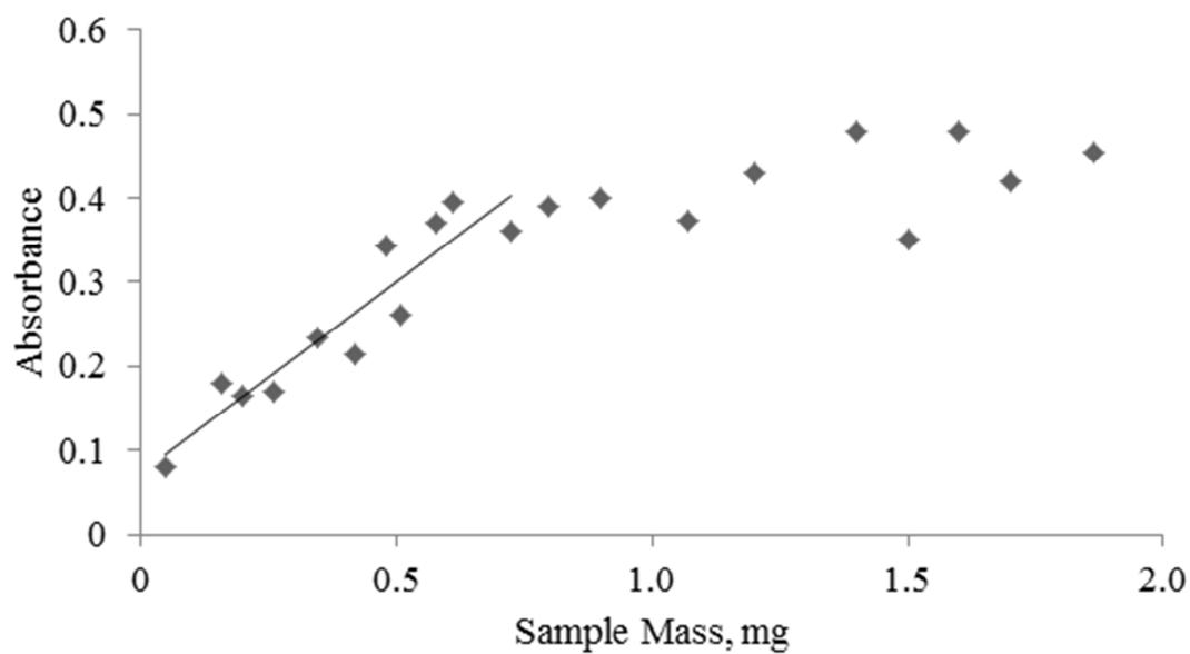
Figure 2: The effect of sample mass on the sensitivity of lead.
