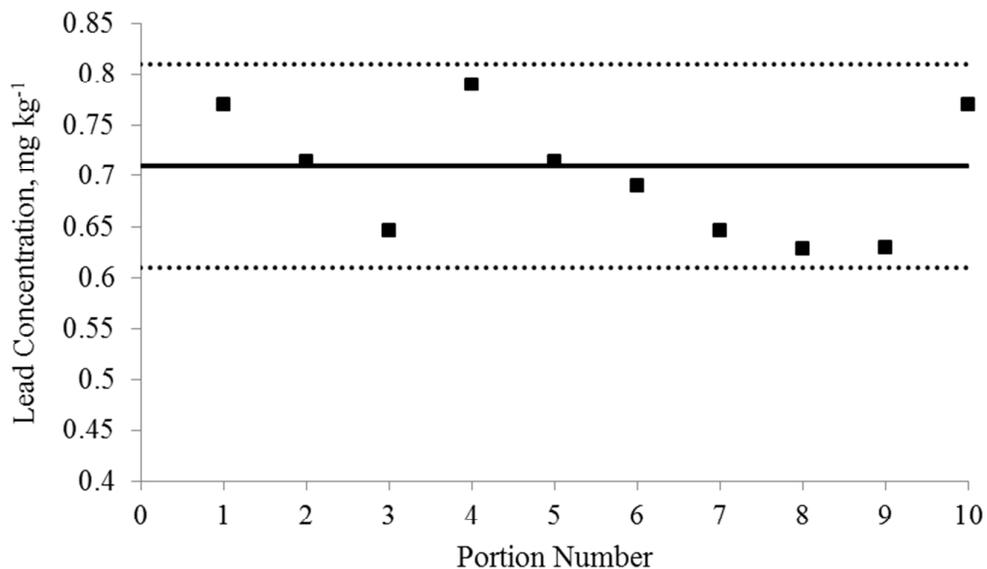
Figure 3. Distribution of lead concentrations in different sample portions of a PVC toy sample. (solid horizontal line is the mean concentration; dotted lines are 3SD values of measurements)
