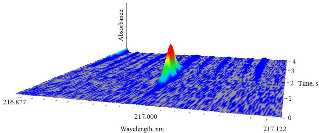
Figure 1: Time and wavelength resolved (3D) absorption spectrum of a plastic sample in the vicinity of 217.005 nm obtained according to graphite furnace program given in Table 1 and in the presence of Pd +Mg modifier.
