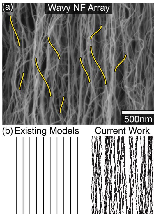
**Fig. 1** Real wavy nanofibers (NFs) and theoretical frameworks. (a) Representative high resolution scanning electron microscopy image of wavy arrays of NFs, specifically carbon nanotubes. (b) Illustration of the NF morphology normally assumed in existing theoretical frameworks, which neglect the NF waviness, and the wavy NFs with realistic stochastic morphologies generated using the simulation framework presented here.
