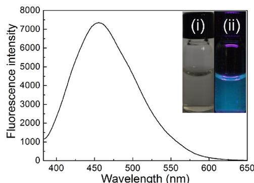
Fig. 2 The fluorescence emission spectrum of the trypsin-stabilized CuNCs with the excitation wavelength of 363 nm. Inset: the photographs of the 20-fold diluted trypsin-stabilized CuNCs under the visible light (i) and 365 nm UV light irradiation (ii), respectively.
