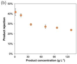
Fig. 7 (a) The average catalyst and product rejection in each diafiltration cycle. Inset: photo of the Borsig oNF-1 membrane coupon after five cycles of catalyst reuse experiments. (b) The rejection of Stage 2 product at varying product concentrations. The feed solution was prepared by diluting the Stage 2 reaction mixture with 2-MeTHF to the desired concentration.
