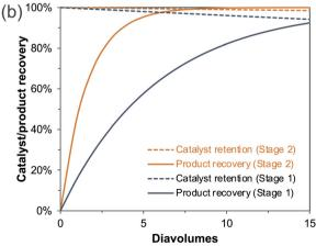
Fig. 3 (a) The rejection of Borsig oNF-1 (600 Da) towards catalyst and product in Stage 1 vs. Stage 2, (b) the comparison of the calculated catalyst retention and product recovery during diafiltration in Stage 1 vs. Stage 2.
