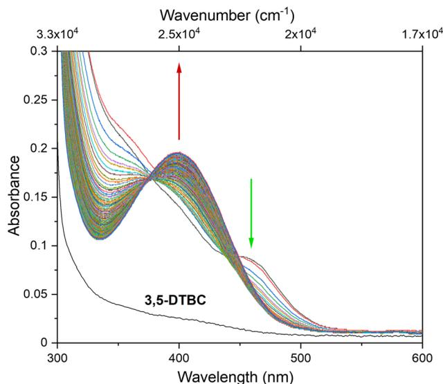
**Fig. 12** UV-vis spectra recorded during the oxidation reaction of 3,5-DTBC catalysed by complex **1** in CH<sub>3</sub>CN. Spectra were collected in the first 20 min of the reaction, just after addition of the solution of **1** to the 3,5-DTBC solution, with 2 s intervals ([3,5-DTBC] =  $7.4 \times 10^{-3}$  M and [Cat] =  $5 \times 10^{-5}$  M).
