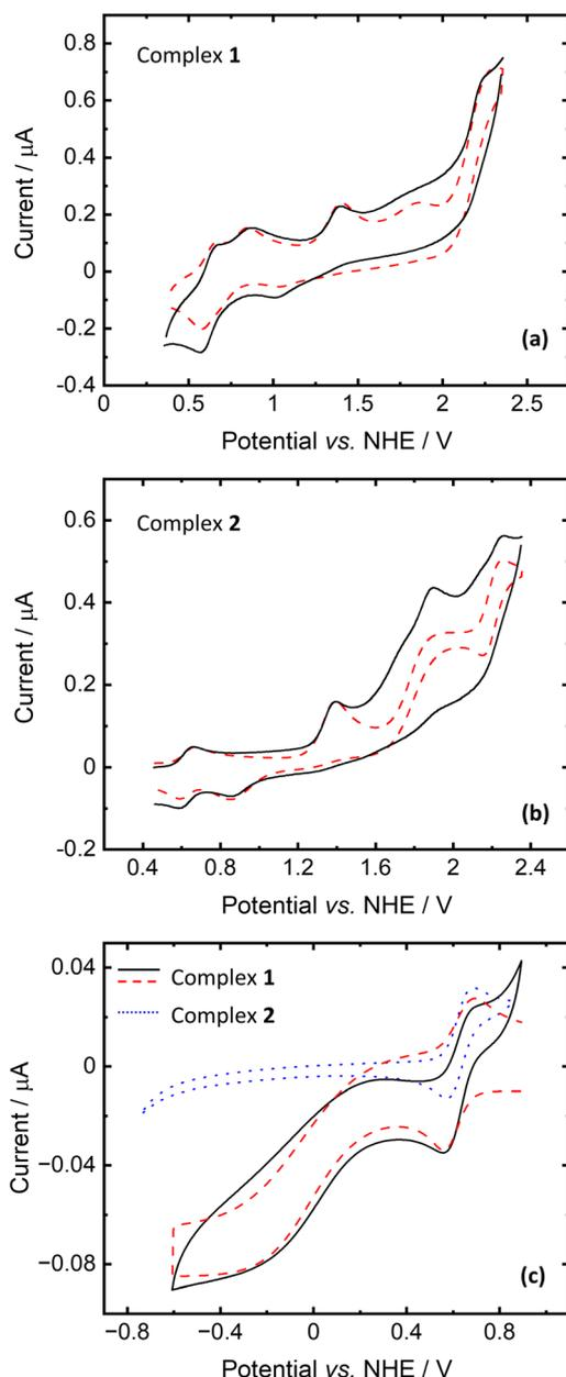
**Fig. 8** Cyclic voltammograms of complexes **1** and **2** (each at a concentration of 1 mM) recorded under an ambient air atmosphere in  $\text{CH}_3\text{CN}$  solution containing 0.1 M  $\text{NBu}_4\text{PF}_6$  with the scan rates of  $10 \text{ V s}^{-1}$  and  $1 \text{ V s}^{-1}$  for oxidation and reduction, respectively. Lines (—) and (---) represent the experimental and simulated curves, respectively.
