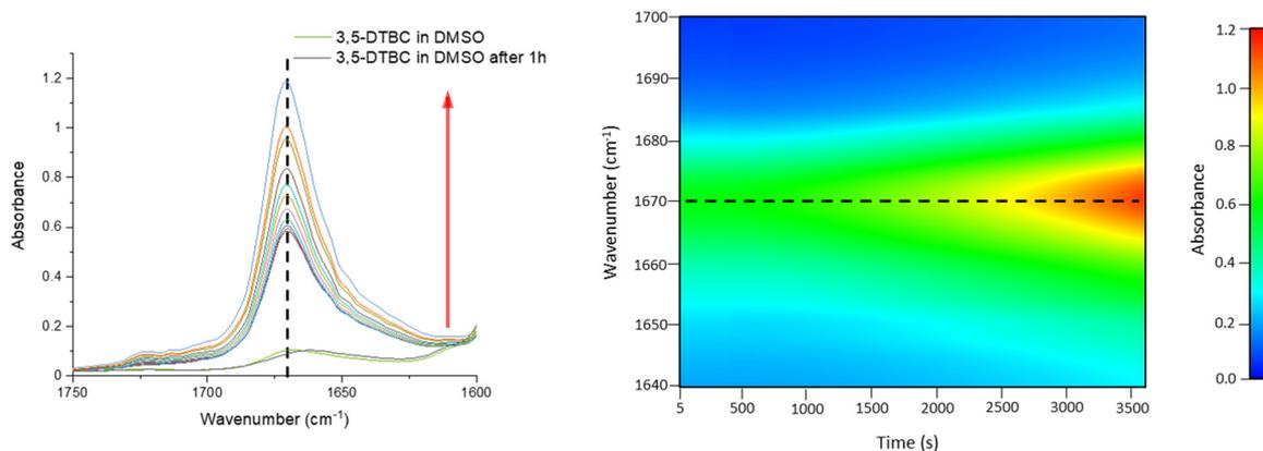
**Fig. 10** Changes in the FT-IR spectrum in the 1750–1600  $\text{cm}^{-1}$  region (5 min intervals) and 2D contour map recorded after addition of catalyst **1**, during the first hour of oxidation of 3,5-DTBC ( $1 \times 10^{-1}$  M) to the corresponding quinone in the presence of **1** ( $1 \times 10^{-3}$  M) in DMSO.
