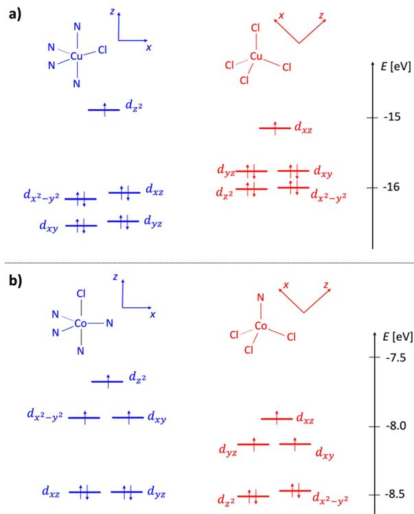
**Fig. 4** Molecular orbital diagrams of complexes **1** (a) and **2** (b). Cationic fragments are shown in blue and anionic in red. The energy scale corresponds to the eigenvalues of alpha molecular orbitals in an unrestricted treatment ( $\omega$ B97X/DKH-def2-TZVP level).
