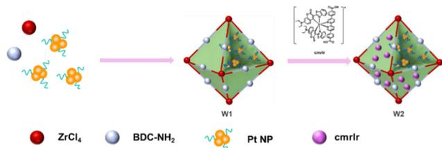
Fig. 1 Scheme for the preparation of cmrIr/Pt@UiO-66-NH<sub>2</sub>.
