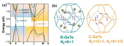
Fig. 9 (a) Calculated electronic band structure of GeTe featuring both R-GeTe (rhombohedral GeTe) and C-GeTe (cubic GeTe) respectively; (b) calculated Fermi surfaces for both R-GeTe and C-GeTe considering spin-orbit coupling. Reproduced and reprinted from ref. 45, © 2020 Wiley-VCH Verlag GmbH & Co. KGaA, Weinheim.
