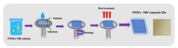
Scheme 1 Fabrication of PMMA-NBF:Gd/Tb composite films.
