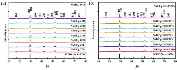
Fig. 1 Powder XRD patterns of (a) NBF:x%Tb and (b) NBF:20%Gd,x%Tb
