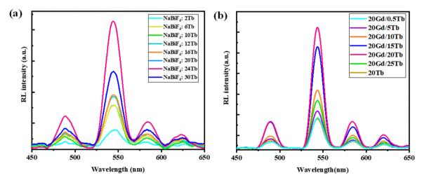
Fig. 4 (a) RL spectra of NBF:Tb and (b) NBF:20%Gd,Tb (x = 0.5-25%) nanoparticles.
