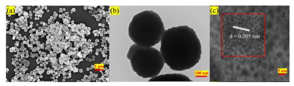
Fig. 2 (a) FE-SEM, (b) TEM and (c) HRTEM images of the NBF:Gd,Tb nanoparticles.
