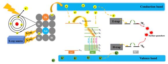
Fig. 6 Proposed energy conversion and transport and luminescence mechanisms in the NBF:Gd/Tb nanoscintillator.
