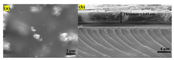
Fig. 7 (a) FESEM image of a PMMA-NBF film and (b) cross-sectional FE-SEM image of a PMMA-NBF thin film.
