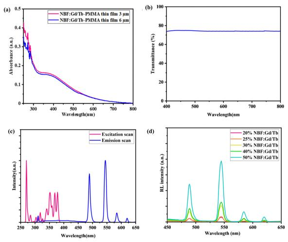
Fig. 8 (a) Absorption spectra of PMMA–NBF films of thickness 3 and 6 μm; (b) transmission spectra of the PMMA–NBF film; (c) excitation and PL spectra of the PMMA-NBF film; (d) XEOL spectra of PMMA-NBF with different loading percentages.
