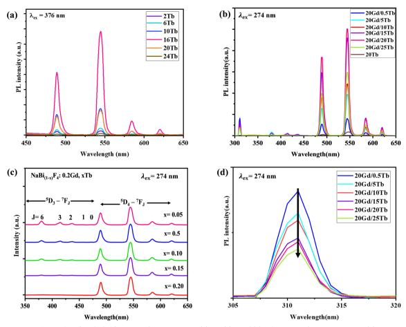
Fig. 3 (a) PL spectra of NBF:x%Tb (x = 2-24%) under 376 nm excitation; (b) and (c) NBF:20Gd,x%Tb under 273 nm excitation; (d) PL emission spectra from Gd<sup>3+</sup> ions corresponding to emission at 310 nm.
