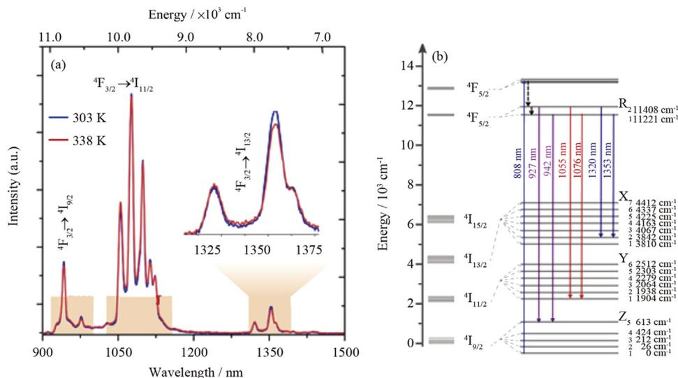
Fig. 4 (a) NIR emission spectra of  $(\text{Gd}_{0.98}\text{Nd}_{0.02})_2\text{O}_3$  NPs in Dulbecco's modified Eagle's medium at 25 and 65 °C. The shaded regions depict 1<sup>st</sup>, 2<sup>nd</sup> and 3<sup>rd</sup> BWs; (b) partial energy level diagram of  $\text{Nd}^{3+}$  ions showing the transitions used for defining the thermometric parameters.<sup>72</sup>
