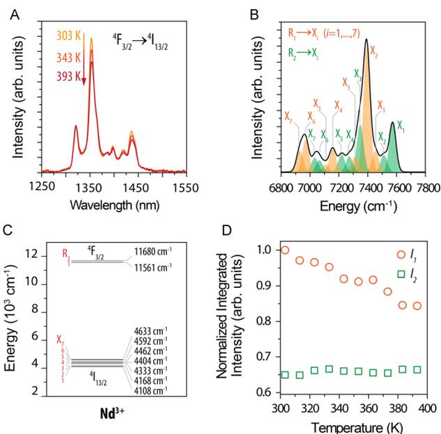
Fig. 5 (A) Part of emission spectra of  $(\text{Gd}_{0.972}\text{Nd}_{0.028})_2\text{O}_3$  NPs recorded in the 30–120 °C (303–393 K) range under 808 nm excitation. (B) Deconvoluted emission spectrum obtained at 50 °C (323 K). (C) Simplified energy level diagram. (D) Normalized integrated intensity of  $I_1$  (orange circles) and  $I_2$  (green squares). Reprinted from ref. 90; Copyright (2016), with permission from Elsevier.
