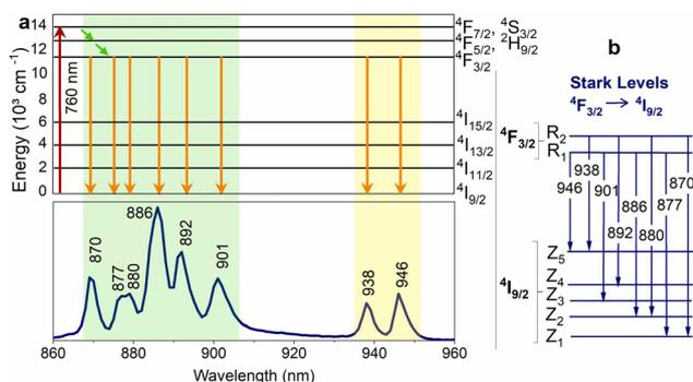
Fig. 3 (a)  $\text{Nd}^{3+}$  partial energy level diagram illustrating the excitation (760 nm) and relaxation pathways. The bottom part of the figure shows the corresponding emission spectrum of  $\text{Y}_3\text{Al}_5\text{O}_{12}:\text{Nd}^{3+}$  NPs. (b) Representation of the Stark levels of the  $\text{Nd}^{3+}$  manifolds  ${}^4\text{F}_{3/2}$  and  ${}^4\text{I}_{9/2}$ , as well as the electronic transitions associated with the emission peaks in the lower part of Fig. 3a.<sup>82</sup>
