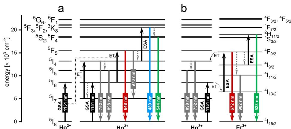
Fig. 9 The mechanism of upconversion in the (a) NaYF<sub>4</sub>:Ho<sup>3+</sup>@NaYF<sub>4</sub> and (b) NaYF<sub>4</sub>:Ho<sup>3+</sup>, Er<sup>3+</sup>@NaYF<sub>4</sub> NPs observed under 1151 nm excitation.<sup>113</sup>
