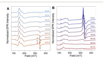
Fig. 3 CW EPR spectra ( $\nu=9.37$  GHz,  $P_{\mu\nu}=20$  mW) of (A) NiFd-CN and (B) NiFd-CO at the indicated temperatures. Spectra were normalized to temperature using a standard Curie dependence [ $I \times T$ ]. \* denotes small (<5%) amount of contaminating S=1/2 [Fe<sub>4</sub>S<sub>4</sub>]-CN Fd.
