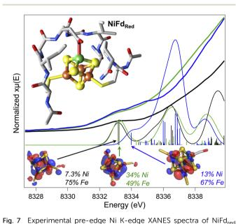
(green), NiFd<sub>ox</sub> (black), and NiFd-CO (blue) with calculated TD-DFT contributions using the DFT geometry-optimized structures of the NiFd species (inset). Dominant contributing orbital to the indicated transition for each species shown at an isosurface value of 0.03 with distribution over Ni and the Fe atoms indicated.
