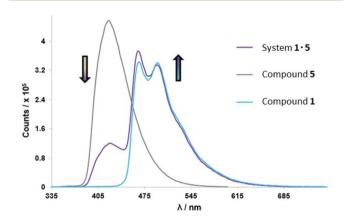
Fig. 7 Overlaid emission spectra of complex 1 (blue), compound 5 (grey) and co-complex  $1\cdot 5$  (purple) from FRET studies in CHCl<sub>3</sub> solution. All samples excited at  $\lambda_{\rm ex}=350$  nm.
