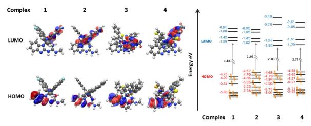
Fig. 5 (left) TD-DFT predicted HOMO and LUMO orbital distributions of complex 1–4 and (right) visualisation of the energy levels of frontier orbitals with computationally obtained HOMO–LUMO gap.
