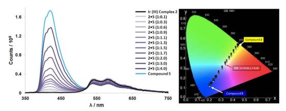
Fig. 8 (left) Emission spectra from titration studies of complex 2 with additions of compound 5 measured in  $CHCl_3$  solution. Black line represents emission of iridium complex 2 without any additions, blue line represents compound 5 with no complex 2 present. (right) CIE diagram from emission titration experiment of host complex 2 and guest compound 5.
