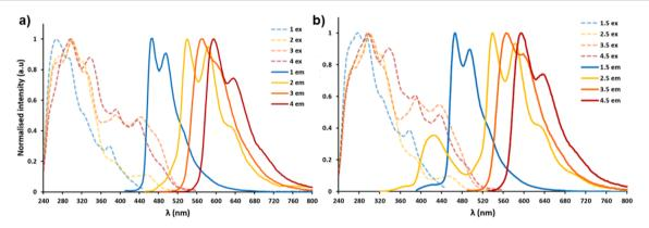
Fig. 4 (a) The normalised absorption–emission spectra of complex 1–4, dashed line representing the excitation of each complex and solid line representing the emission, all spectra were measured in CHCl<sub>3</sub> ( $1.0 \times 10^{-5}$  M). (b) The normalised absorption–emission spectra of complex 1–4 with compound 5 in a 1:1 molar ratio in CHCl<sub>3</sub> ( $1.0 \times 10^{-5}$  M).
