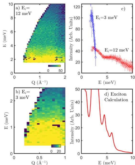
**Fig. 3** Summary of the neutron spectroscopy results taken on LET at  $T = 2$  K with background and phonon corrected data displayed in (a)  $E_i = 12$  meV and (b)  $E_i = 3$  meV. (c) Momentum integrated intensity normalized at  $E = 2.5$  meV for  $E_i = 3$  meV ( $\vec{Q} = [0, 1] \text{ \AA}^{-1}$ ) and  $E_i = 12$  meV ( $\vec{Q} = [0, 2] \text{ \AA}^{-1}$ ). (d) Excitonic calculation described in the main text constrained by first principles calculations.
