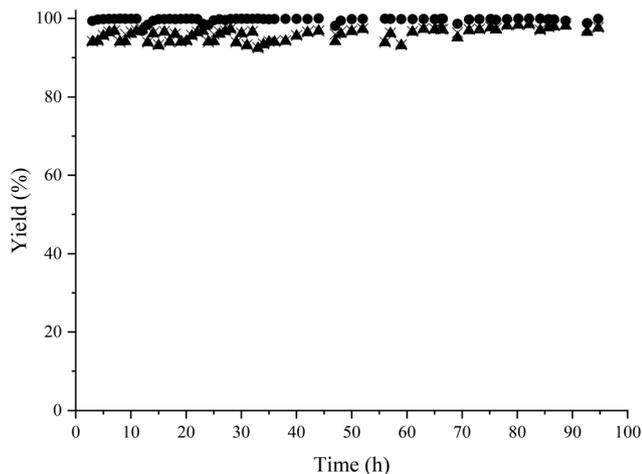
**Fig. 6** Results of the reductive amination of HMF with methylamine in a continuous-flow reactor using Co@C NPs as a catalyst. Reaction conditions: HMF in 2-MTHF (3.5 wt%), methylamine (2 M in THF) (1.2 equivalents regarding HMF), 300 mg of catalyst, flow rate 1.32 mL h<sup>-1</sup> (WHSV: 0.13 h<sup>-1</sup>) at 60 °C and 4 bar of H<sub>2</sub>, hydrogen flow 29 mL h<sup>-1</sup>. HMF conversion (▲); amino-alcohol 5 yield (●); amino-alcohol selectivity (x).
