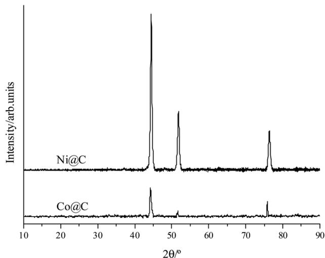
Fig. 1 XRD patterns of Co@C and Ni@C nanoparticles.
