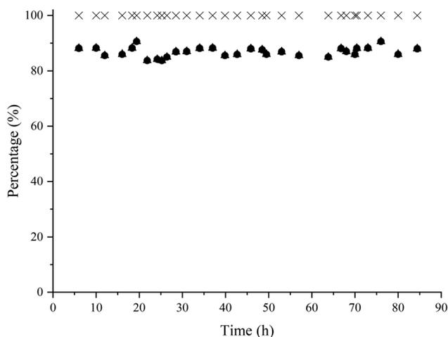
**Fig. 8** Results of the bioesterification of the amino-alcohol 5 with hexanoic acid in a continuous-flow reactor using Novozym 435 as a catalyst and molecular sieves. Reaction conditions: amino-alcohol 5 in 2-MTHF feed (0.28 wt%), hexanoic acid (0.9 wt%), Novozym 435 (50 mg), molecular sieves 4 A 0.4–0.6 mm (2.4 g), flow rate 1 mL h<sup>-1</sup> (WHSV: 0.045 h<sup>-1</sup>) at 35 °C. Amino-alcohol 5 conversion (▲); amino-ester 6 yield (●); selectivity to 6 (x).
