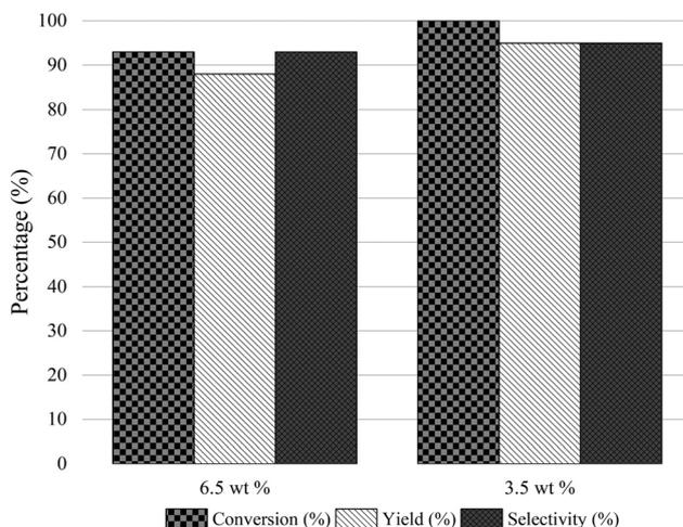
**Fig. 5** Optimization of the contact time in the flow reactor for the reductive amination of HMF with methylamine. Reaction conditions: HMF in 2-MTHF feed (6.5 and 3.5 wt%, respectively), at 60 °C, at a flow rate of 1.32 mL h<sup>-1</sup>, at 4 bar of H<sub>2</sub> and at a hydrogen flow of 29 mL h<sup>-1</sup>.
