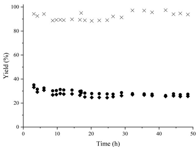
**Fig. 7** Study of the catalyst stability in the reductive amination of HMF with methylamine in a continuous-flow reactor using Co@C NPs as a catalyst. Reaction conditions: HMF in 2-MTHF (3.5 wt%), 150 mg of catalyst, flow rate 11.1 mL h<sup>-1</sup> (WHSV: 2.22 h<sup>-1</sup>) at 60 °C and 4 bar of H<sub>2</sub>, hydrogen flow 29 mL h<sup>-1</sup>. HMF conversion (▲); amino-alcohol 5 yield (●); amino-alcohol selectivity (x).
