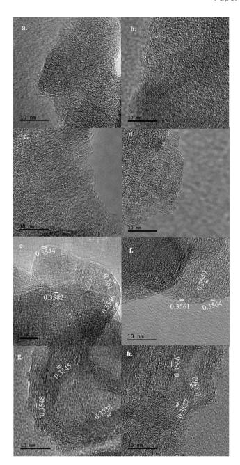
Fig. 4 TEM images of 100% OL-derived CFs. (a) NCF700; (b) NCF800; (c) NCF900; (d) NCF1000; (e) TCF700; (f) TCF800; (g) TCF900; (h) TCF1000.
