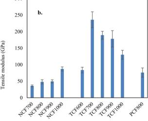
Fig. 3 Tensile properties of CFs produced using 100% OL using different processing conditions. (a) Tensile strength; (b) tensile modulus.
