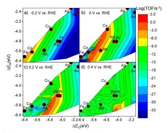
Fig. 5 Theoretical volcano plots of the TOF as a function of atomic oxygen ( $\Delta E_{\rm O}$ ) and nitrogen ( $\Delta E_{\rm N}$ ) adsorption energies for electrocatalytic nitrate reduction on transition metal surfaces based on DFT-based microkinetic simulations at (a) -0.2 V, (b) 0 V, (c) 0.2 V, and (d) 0.4 V vs. RHE by Liu et al. Reprinted with permission from ref. 52. Copyright 2019, American Chemical Society
