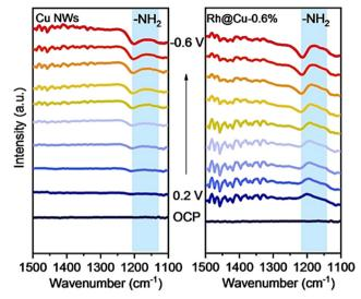
Fig. 13 Electrochemical in situ infrared spectroscopy (IR) of Rh@Cu-0.6% and Cu NWs under different potentials in a 0.1 M Na<sub>2</sub>SO<sub>4</sub> electrolyte (pH 11.5) with 0.1 M KNO<sub>3</sub> by Liu et al. Reprinted with permission from ref. 83 Copyright 2022 Wiley-VCH GmbH.
