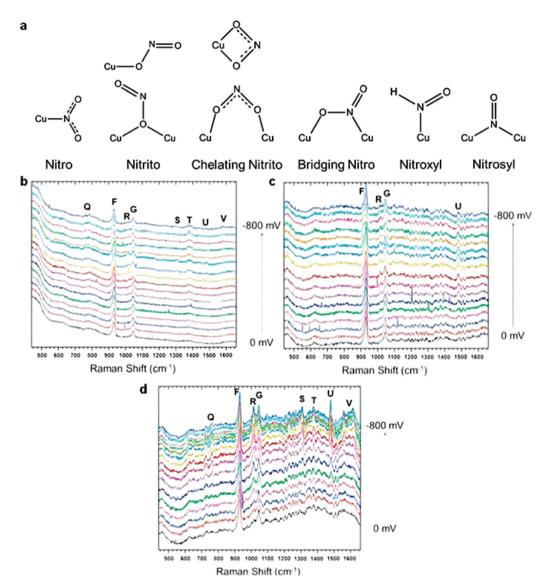
Fig. 15 (a) Adsorption modes of nitrite, nitric oxide, and HNO on the Cu surface. Electrochemical *in situ* SHINERS spectra collected from (b) Cu (100), (c) Cu (111), and (d) Cu (110) in a 0.1 M HClQ<sub>4</sub> solution with 0.05 M HNO<sub>3</sub> and 10 mM HCl at a potential between 0 and -0.8 V vs. Ag/AgCl. Reprinted with permission from ref. 157 Copyright 2016 Elsevier Ltd.
