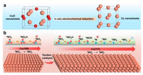
Fig. 9 Schematic illustration for enhancing the electrochemical NO<sub>3</sub>RR over Cu nanosheets via tandem catalysis. (a) Electrochemical in situ reduction of the as-prepared CuO nanosheets during NO<sub>3</sub>RR. (b) Tandem interaction of Cu (100) and Cu (111) facets. Reprinted with permission from ref. 100. Copyright 2023 Wiley-VCH Verlag GmbH
