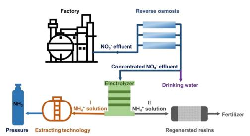
Fig. 18 The schematic illustration of the practical application of nitrate-to-ammonia conversion from wastewater. Reprinted with permission from ref. 50 Copyright 2020 Wiley-VCH.
