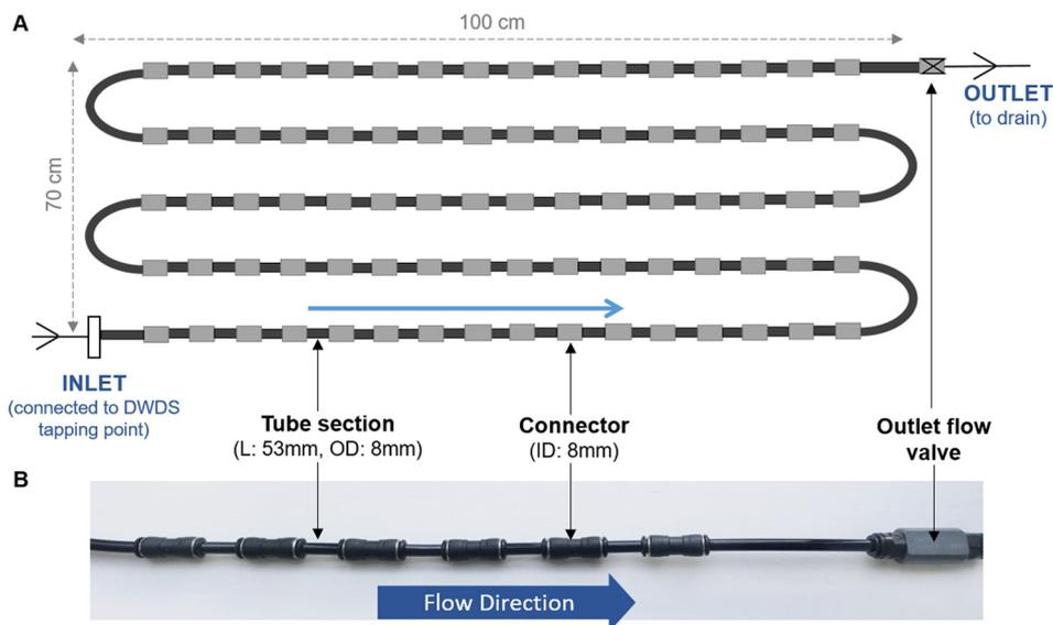
**Fig. 1** Biofilm monitoring device (BMD) schematic (A) and image (B).  $L$  = length; OD = outside diameter, ID = inner diameter, blue arrows indicate direction of water flow. (A) Schematic showing installation of five rows of the BMD (row  $L$  = 100 cm, height of all rows = 70 cm, total  $L$  ~ 500 cm). Note schematic does not show the full number of pipe sections used in an installation. (B) Photo of short section of BMD *in situ*.
