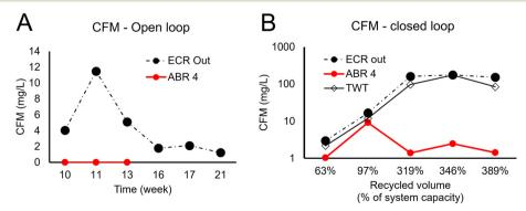
Fig. 6 DPB chloroform (CFM) generation. (A) Open loop at different field testing timepoints; ECR out: electrochemical reactor after treatment; (B) closed loop from three sampling points (ABR4, ECR out, treated water tank (TWT)), with measurements carried at different stages of recycled volume
