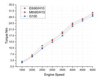
Fig. 4 Effect of varying speeds on torque using hydrogen-blended methanol and ethanol alternative fuels, with gasoline 100%.
