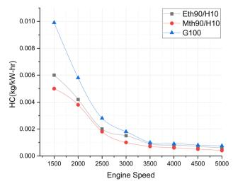
Fig. 8 Effect of varying speeds on hydrogen emissions using hydrogen-blended methanol and ethanol alternative fuels, with gasoline 100%
