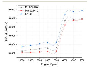
Effect of varying speeds on NOx emissions using hydrogenblended methanol and ethanol alternative fuels, with gasoline 100%.
