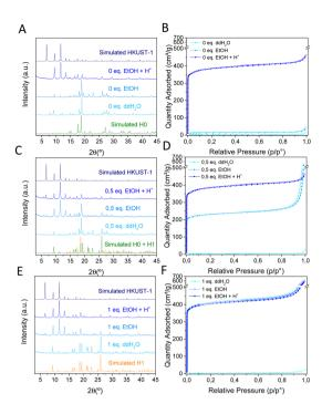
Fig. 1 XRPD patterns (left) and N<sub>2</sub> sorption isotherms (right) of Cu-BTC materials synthesized with (A, B) 0 equivalents, (C, D) 0.5 equivalents and (E, F) 1 equivalent of HCl and the corresponding products washed with water (ddH2O), ethanol (EtOH) or ethanol and acid (EtOH + H+). H0: CCDC 609754,11 H1: CCDC 1288676.12
