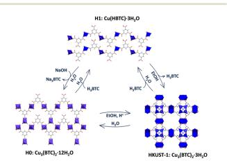
Fig. 2 Schematic representation of the reversible transformation processes among the different Cu-BTC phases.
