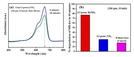
Fig. 8 (a) Absorbance spectra of MB dye using 0.3 g of TiO<sub>2</sub> (non-piezoelectric material) in 60 min with ball milling at 200 rpm using 10 balls, (b) % degradation of MB dye in 60 min using 0.3 q of BaTiO<sub>3</sub>, TiO<sub>2</sub>, and without using any catalyst in 60 min with ball milling at 200 rpm using 10 balls.
