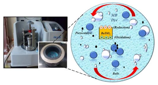
Schematic representation of piezocatalysis process induced from ball milling for MB dve degradation.
