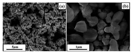
Fig. 2 SEM images of synthesized BaTiO<sub>3</sub> at a resolution scale of (a) 5  $\mu$ m, (b) 1  $\mu$ m.
