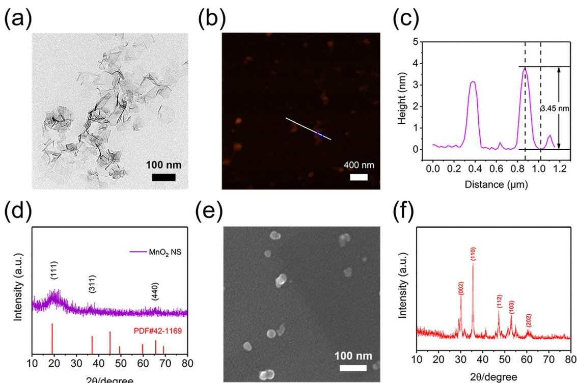
Fig. 1 Characterization of MnO<sub>2</sub> NS and CaO<sub>2</sub> NPs. (a) TEM image of MnO<sub>2</sub> NS. (b) AFM image and (c) the corresponding height image of MnO<sub>2</sub> NS dispersed on a mica substrate. (d) XRD patterns of bulk  $\delta$ -MnO<sub>2</sub> and MnO<sub>2</sub> NS. (e) SEM image and (f) XRD pattern of CaO<sub>2</sub> NPs.
