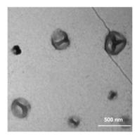
Fig. 7 TEM image of structures made from mixing 1.5 μM mCherry-Z<sub>E</sub> and 30  $\mu$ M Y<sub>5</sub>-Z<sub>R</sub>-ELP at 0.15 M NaCl and warming from 4 to 25  $^{\circ}$ C for one hour
