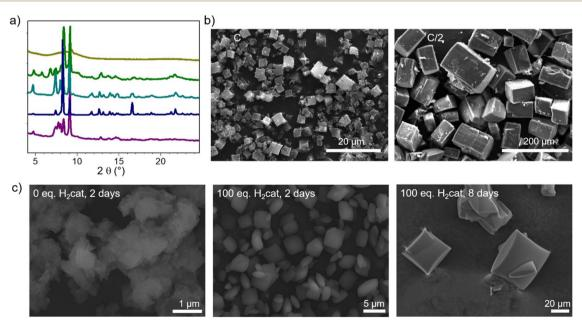
Fig. 3 (a) PXRD patterns of the samples synthesized in various solvents; from top to down: pure DEF, DEF/ $H_2O = 3$ , DEF/ $H_2O = 1$ , and DEF/ $H_2O = 1$ . = 1 and concentration lowered twice, DEF/H<sub>2</sub>O = 1/3; (b) SEM images of CatPMOF-2(Al): effect of the concentration of reactants; (c) SEM images of Ni-CatPMOF-2(Al): effect of the amount of  $H_2$ cat and reaction time ( $H_{10}$ TcatPP/AlCl<sub>3</sub> = 1/2, DEF, and 160 °C).
