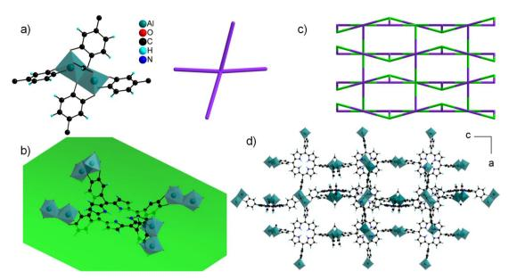
Fig. 8 Crystal structure of CatPMOF-2(Al). (a) Inorganic SBU (left) acting as a distorted square planar node (right); (b) H<sub>2</sub>TcatPP ligand, with the mean plane of the macrocycle shown in green; (c) cds net (the ligand and the inorganic SBU are shown in green and violet, respectively); (d) full structure shown along the b axis.
