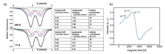
(a) Mössbauer spectra of CatPMOF-1(Fe)-pz at 330 and 77 K and the respective deconvolutions; (b) EPR spectra of CatPMOF-1(Fe)-pz at Fig. 7 120 K
