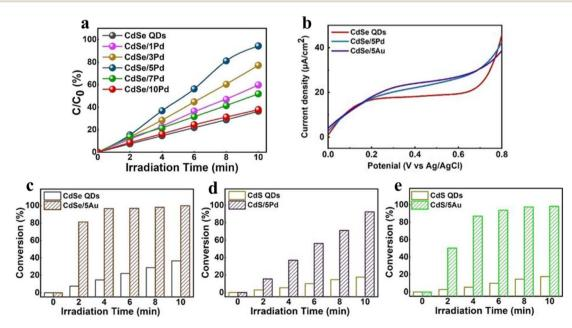
Fig. 6 (a) Photoactivity of selective nitroaromatic reduction over CdSe/Pd nanocomposites with different volume of Pd nanocrystals. (b) LSV plots. Nitroaromatic conversion over (c) CdSe/5Au, (d) CdS/5Pd and (e) CdS/5Au compared to their corresponding single QDs. Reprinted with permission from ref. 75.
