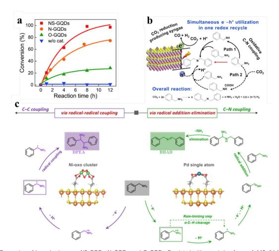
Fig. 12 (a) Conversion of benzylamine over NS-GQDs, N-GQDs, and O-GQDs. Reprinted with permission from ref. 140. (b) Illustration of photocatalytic selective benzylamine oxidation integrated with CO<sub>2</sub> reduction over (BP/ZIS) heterostructures. Reprinted with permission from ref. 141. (c) Mechanism diagram of photocatalytic selective oxidative coupling of benzylamine over different samples. Reprinted with permission from ref. 42.
